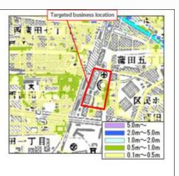
Display of flooded area with mesh size of 10m2 (calculation results)
